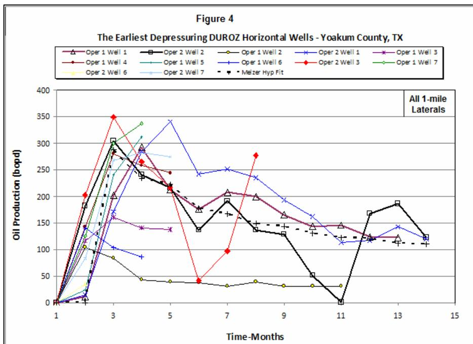
production, we have chosen to curve fit two of the original wells – one from each operator - with a hyperbolic function and use that as our analog well shown in its earliest months in Figure 4.
