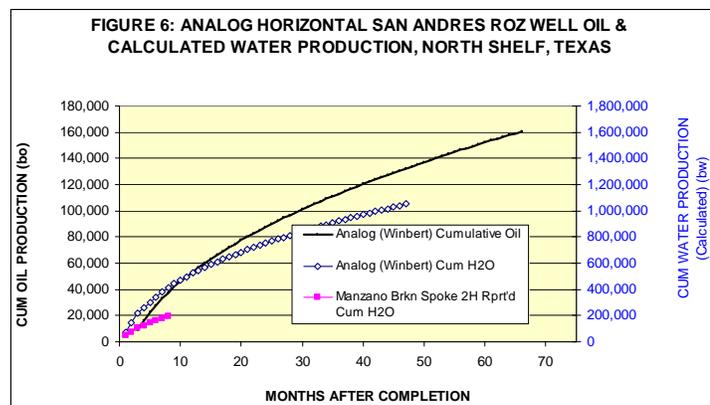
out and remain there for the life of the well. The cumulative oil for the analog well and cumulative water production data is shown in Figure 6 for the wells we have been able to obtain.
